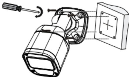
Lead tapping screws through the guide holes in the base and fix them on the wall by using a screwdriver.
