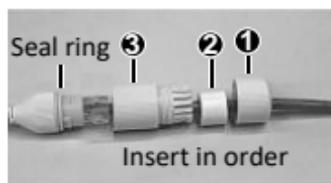
Attach the seal ring to the Ethernet interface. Mount the waterproof components in order. Then insert the cable into the Ethernet interface and screw the waterproof bolt in.
